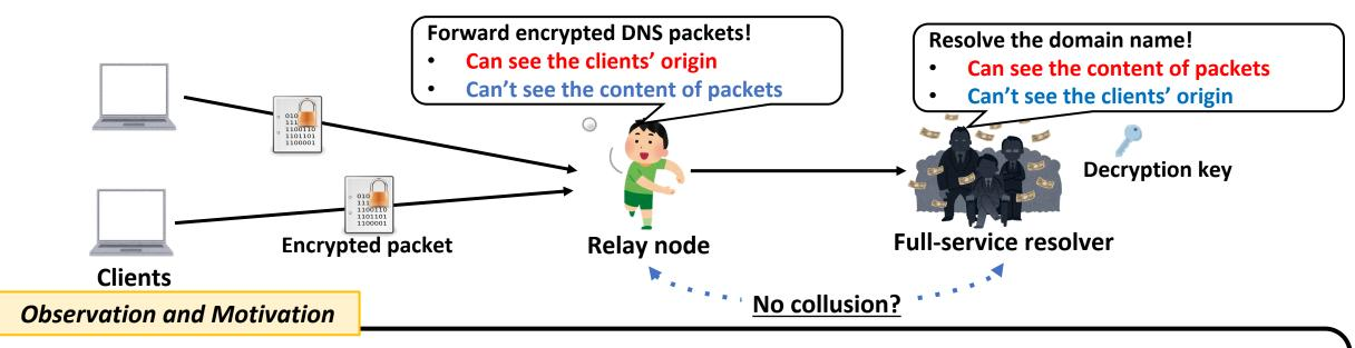
The DNS-dedicated single-relay approach works fast and maintains UX, but is easily corrupted when the relay colludes with the target resolver. (In fact, relay nodes and resolvers typically run by just few big techs.)
