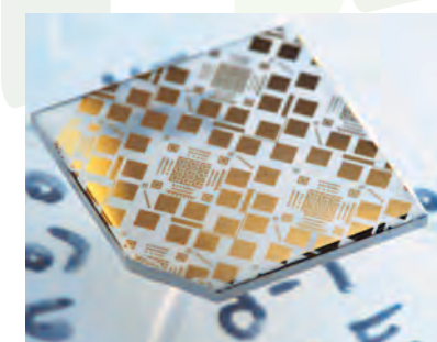
Chip with fabricated Ga 2 O 3 transistors and diodes
