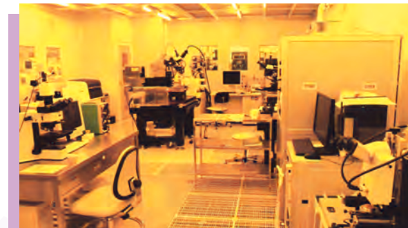
Photo-lithography equipments in the clean room with yellow lights
