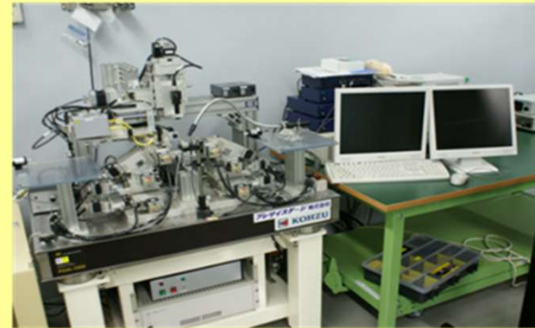
Crosstalk measurement system in asia center
