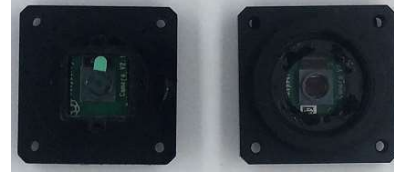
Camera module (V2) L: M12 mount R: CS mount
