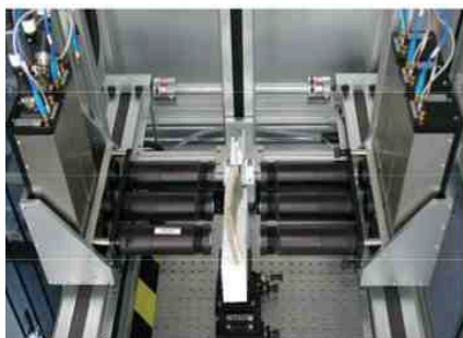
Reflection and transmission setup for flat samples
