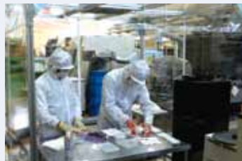
Figure 4●Assembling an LRA in the clean booth at the NICT prototype development building
