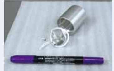
Figure 3●Prism broken during a test
