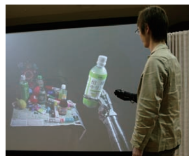
Figure 3 ● Video Image Captured by 4K Robot Vision (Remote-Controlled with 3D Manipulating Gloves)
