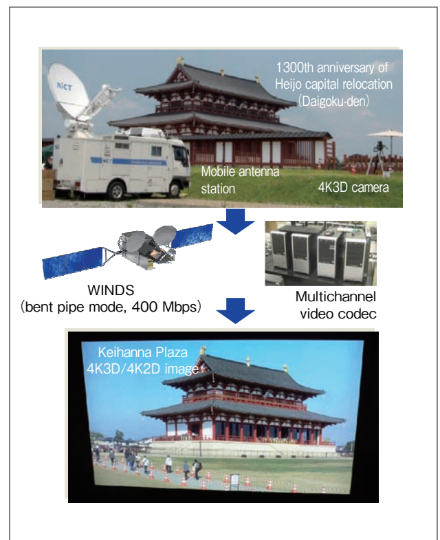
Figure 5 ● 4K3D Live Image Transmission Via WINDS
