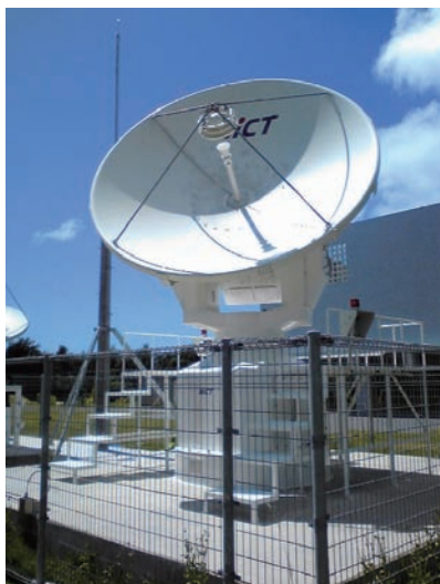
Figure 3 ● 3.7-m Diameter Antenna of Okinawa Station
