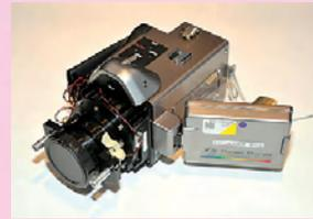
Terahertz camera, innovation in non-destructive inspection
