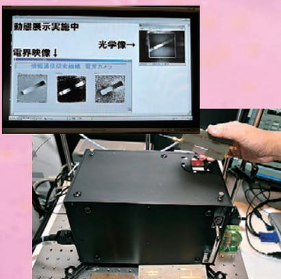
Live electro-optic imaging camera; it provides real-time visual access to the microwave field distributions.
