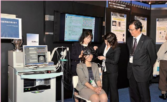
Near-infrared brain-function imaging device capable of measuring how the human brain is working in its natural state
