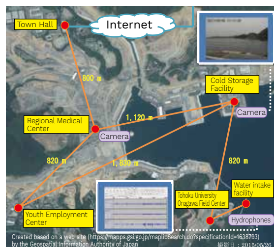
Regional mesh network built in Onagawa
