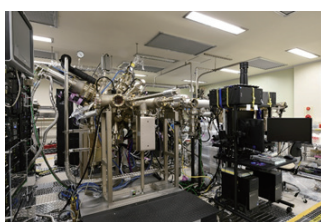
High-quality, semiconductor crystal growth apparatus
