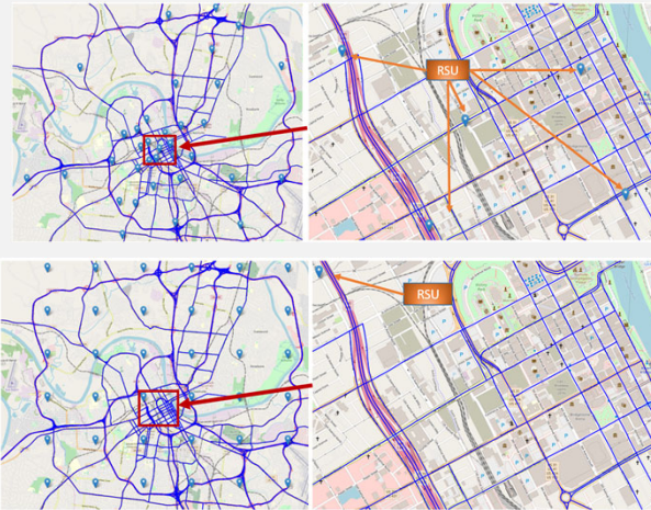
Optimized (for detection) RSU Deployment
