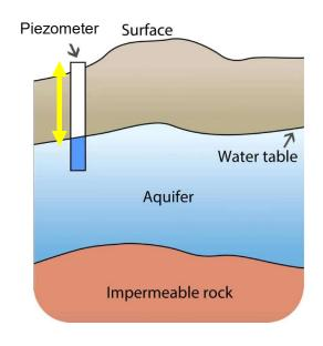
Monitoring water table (level below which the ground is saturated with water)
