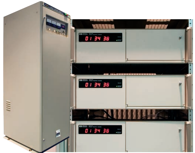
(Left) Hydrogen maser clock (Right) Cesium atomic clock
