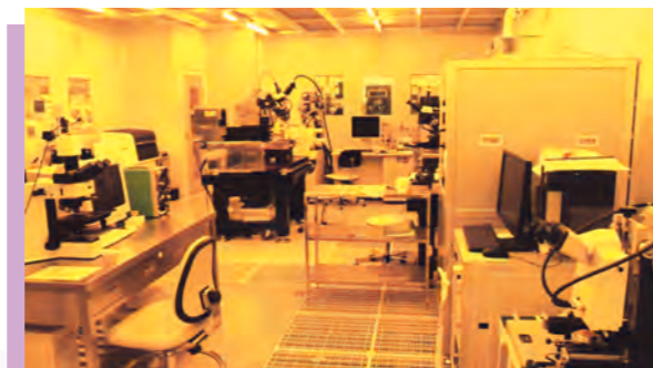
Photo-lithography equipments in the clean room with yellow lights
