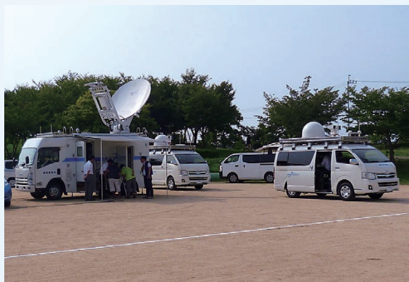
WINDS mobile vehicle earth stations set up at the disaster response headquarters
