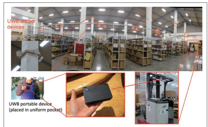
Figure 5 Example of anchor device layout and portable device in distribution warehouse
