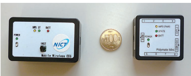
Figure 3 Compact EEG instrument (left), and the instrument for the product based on it (right). To make EEG measurements, electrodes are attached to this instrument and then to the subject's head
