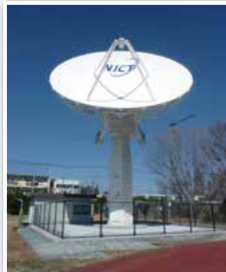
Newly-developed antenna receiving satellite data for solar wind observation
