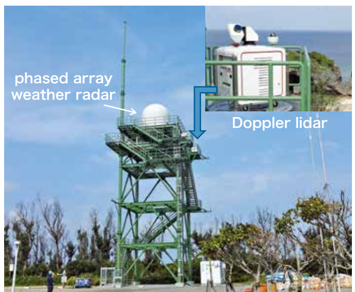
Figure 4 Doppler lidar installed as phased array weather radar-Doppler lidar sensor fusion system in Okinawa
