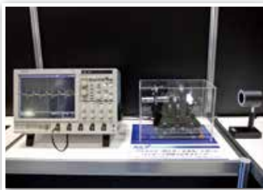
Bipolar differential response light sensor using biomolecules
