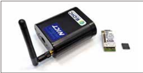
Figure 2 Wi-SUN radio device that supports ECHONET Lite developed in NICT (Left: wireless utility, Right: radio module installed in the radio device)
