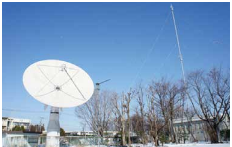
Figure 4 Parabolic antenna inside the premise of NICT for receiving ACE solar wind observation data
