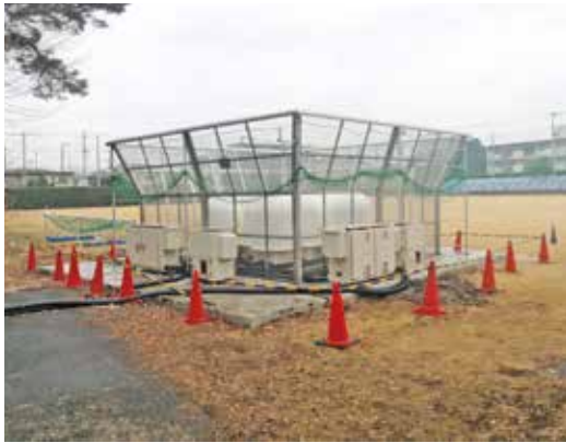
Figure 2 Prototype of next-generation wind profiler (LQ-13)
