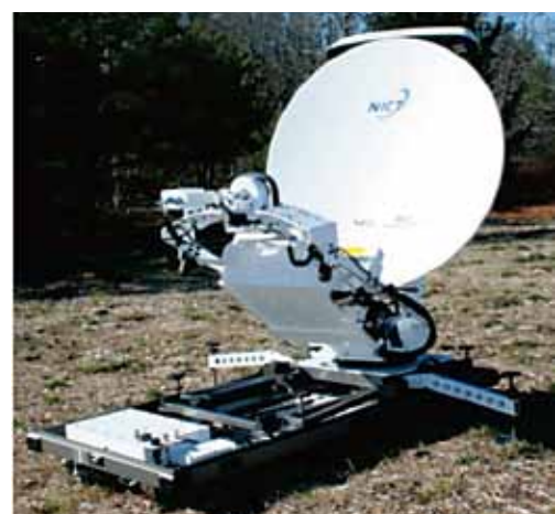
Figure 4 Fully-automatic transportable earth station
