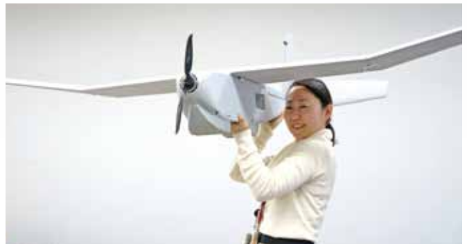
Figure 1 The small unmanned aircraft (Wingspan: 2.8 m, Length: 1.4 m, Weight: 5.9 kg, Flight duration: 2–4 hours, Wind speed: 25 knots, Electric motor, Hand-launch system)
