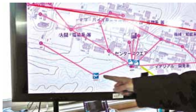
Figure 5 Monitor image showing the communication link between the isolated area and the ground mesh network via the aircraft in real time (the icon the finger is pointing to is an unmanned aircraft relay station)
