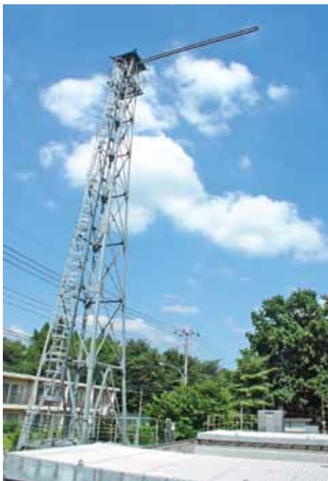
Figure 1 20 m steel tower from where equipment is dropped
