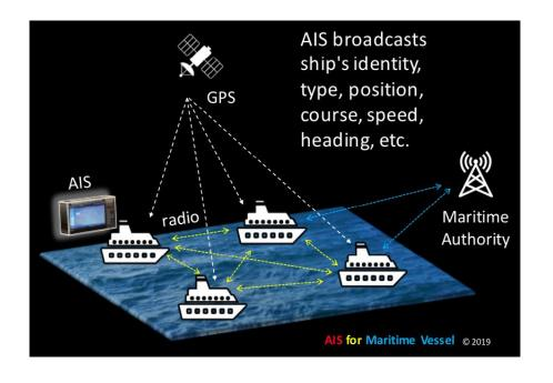
AIS is used for ship-to-ship collision avoidance, ship information gathering, and vessel traffic management. AIS functions by acquiring global positioning system (GPS) coordinates, and exchanging real-time navigation data with other ships and with maritime authorities through the use of radio transmissions.
