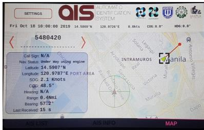
The AIS devices are designed based on international standards, to communicate with one another and with other commercial AIS products. The AIS devices have ship monitoring and tracking tool, that displays the list of nearby vessels, the detailed vessel information, and the location map. The same tool can be installed in the maritime authorities.
