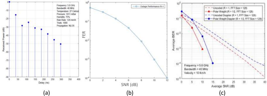
a. Power Delay Profile (PDP) for height of 0-10 m, b. Outage performance, (c) BER with Doppler
