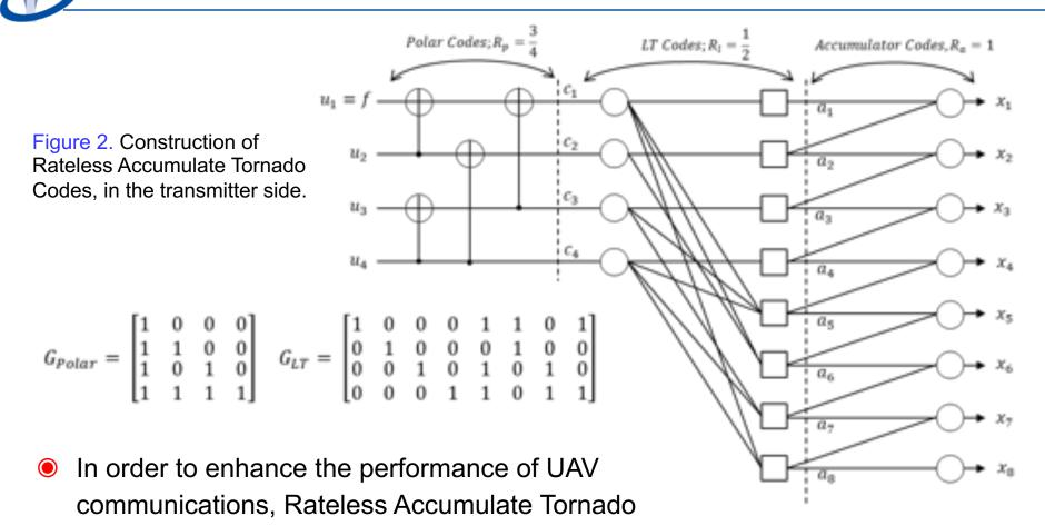
Codes based on Polar-LT-Accumulator Codes will be designed.
