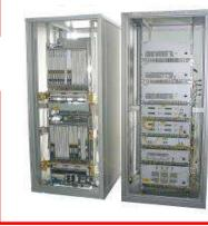
The world's first Optical Packet and Circuit Integrated Network node
