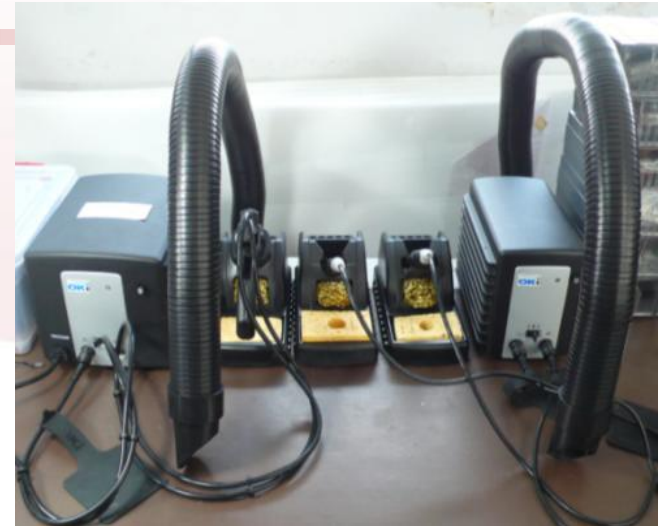
Vacuum Purification Systems
