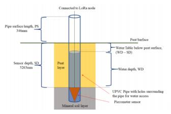
Fig. 3. Piezometer installation layout.
