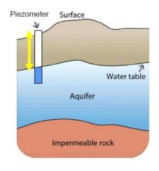
Monitoring water table (level below which the ground is saturated with water)
