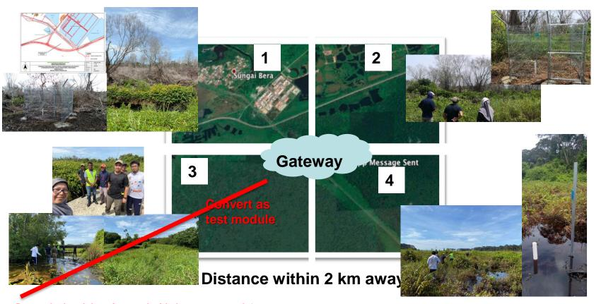
Due to the harsh location we decided to convert node3 as our test module in the lab. If problem exist with any of our 3 other sensors we can replace and fix it without any further downtime.
