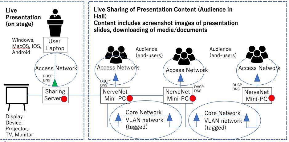
Co-locate Sharing server component with <u>NerveNet</u>. Performance is expected to improve due to nearer access to content/service
