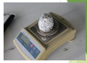
Weighing of Oven Dried Soil Sample
