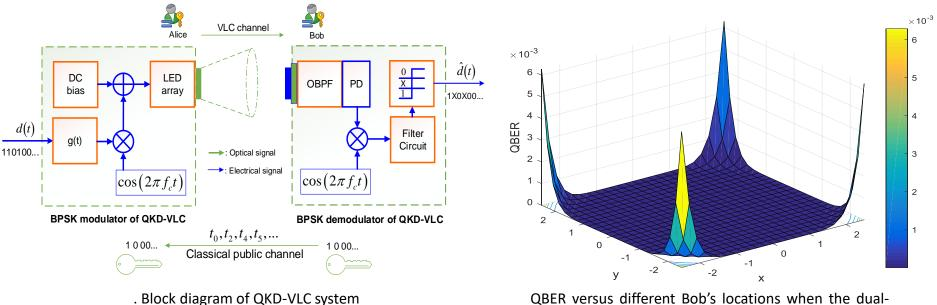
QBER versus different Bob's locations when the dualthreshold scale coefficient  $\delta = 1.5$ , the intensity modulation depth  $\rho = 0.25$  and  $P_{LED} = -3$  dBm
