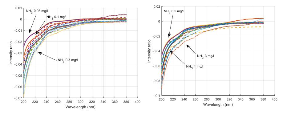
Absorption characteristics of  $NH_3$  from 0.05 mg/l to 3 mg/l
