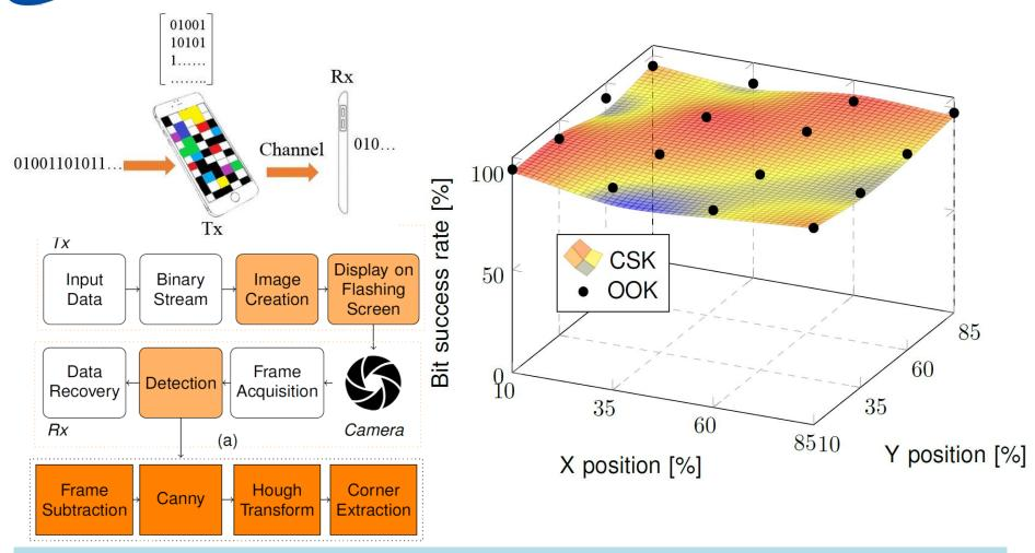
Design and implementation of a complete screen to camera visible light communication system, for smartphones and tablets.
