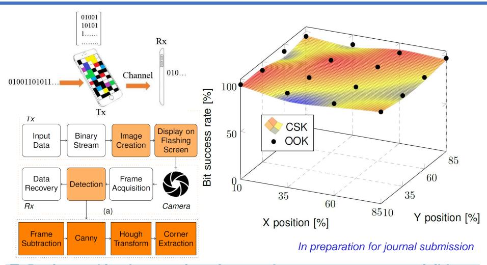
Design and implementation of a complete screen to camera visible light communication system, for smartphones and tablets.
