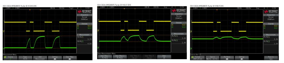
Measured data of transmitting (top) and receiving (below) for 10 mm, 150 mm, and 300 mm.
