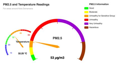
Diagram 1: A Simple Web based dashboard for Air Quality Sensor (source: MIMOS)
