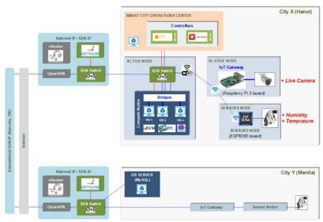
Diagram 3: Experimental Testbed Setup (source and acknowledgement: VNU)
